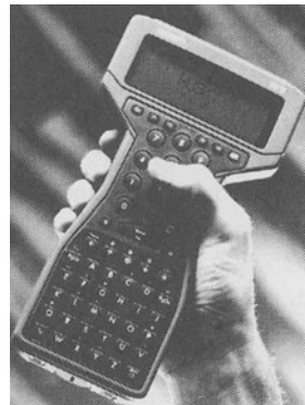
Figure 5.30 Husky Hunter 2 field computer (courtesy Husky Computers Ltd)
