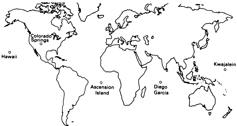
Figure 8.2 GPS control segment
