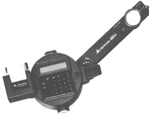
Figure 13.11 Digital planimeter (courtesy Ushikata Mfg. Co. Ltd)
