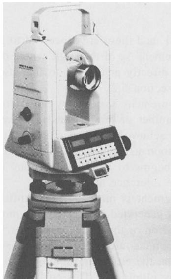
Figure 3.20 Wild T2002 electronic theodolite (courtesy Leica UK Ltd)
