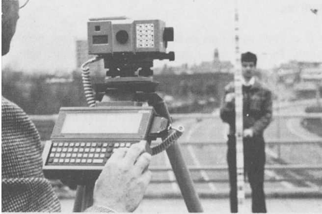
Figure 2.30 Digital level with field computer (courtesy Leica UK Ltd.)
