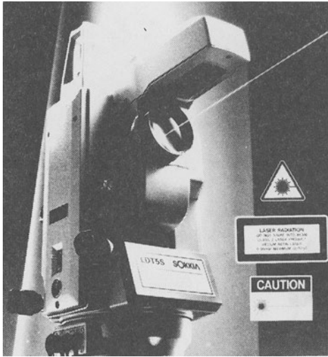
Figure 14.59 Sokkia LDT55 electronic laser digital theodolite (courtesy Sokkia Ltd)
